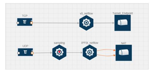
Figure 16: NetFlow on GigaVUE V Series Node on page 77 shows an example of a NetFlow application created on a GigaVUE V Series node in the monitoring session.
