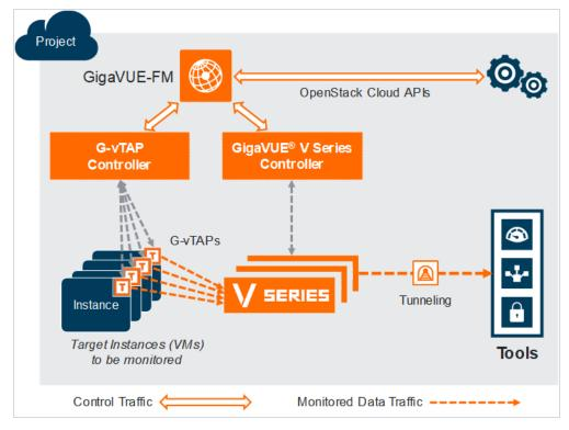
Figure 1: GigaVUE Cloud Components for OpenStack using G-vTAP
